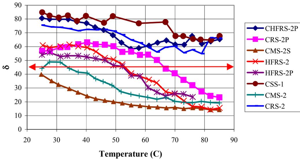
**Figure 6: Temperature Sweep Test ( $\delta$ )**
